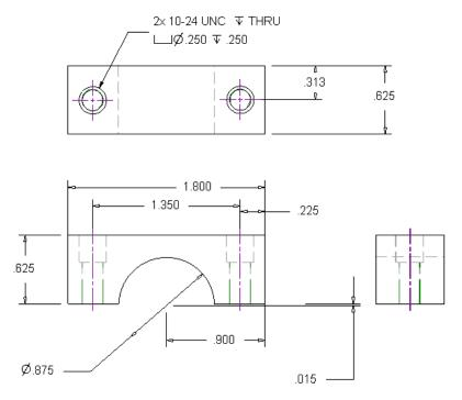
The final step once I am confident that the project is worth drafting up, is to capture the finished design. I am using the Computer Aided Design tool called Alibre here.
