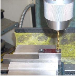
I can now use one of the screws to bolt the clamp block to the support bar. I then put in my #25 drill and move the X axis until it freely goes into the second hole. The clamp block is then swung out of the way and the second hole is made in the support block. I should have started the hole with a centering drill but cheated and just used the #25 drill. It worked OK but is not the best practice. The drill did wander a little before starting to cut.
