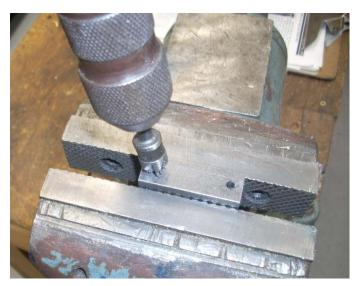
I then use a countersink mounted in a brace and bit to deburr both ends of each hole.
