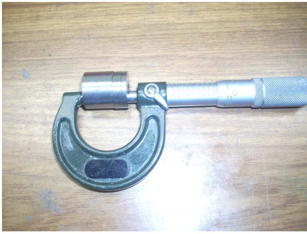
The first step is to mic my spacer stack and record the reading. In this case I found that my mic read 0.0015" over 0.8750". This means that if my mic reads 0.8765" $\Phi$ , my bore is actually 0.8765" - 0.0015" = 0.8750" within the accuracy of the spacer blocks and, more importantly, my skill to measure the bore.
