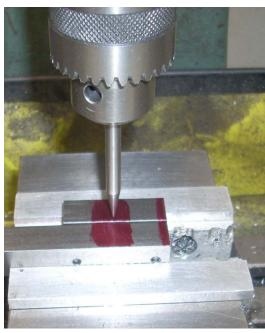
I'm using a pointed length of ¼" rod, called a spud, in my drill chuck. It makes it easy to align the spindle with the center of the hole to be bored out. The X and Y axes are then locked.
