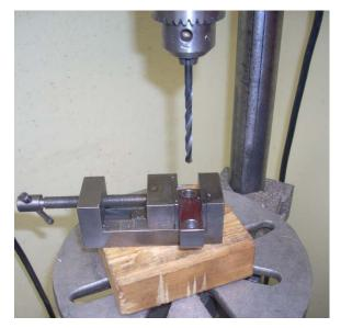
I can now open out the first hole in the clamp block to my clearance diameter. I don't want to disturb my mill so will use my Gingery drill press and homemade vise for the task.
