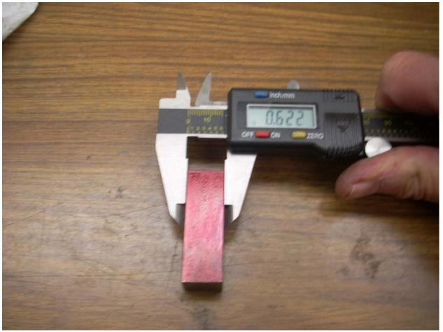
With the clamp block deburred, I first use my red dye on the surface. I then lay out my lines that will locate my two screw holes. To start, I measure the actual width of the block. Minor surprise here. I thought I was using  $\frac{1}{2}$ " bar but it is actually closer to  $\frac{5}{8}$ ". It doesn't really change anything.
