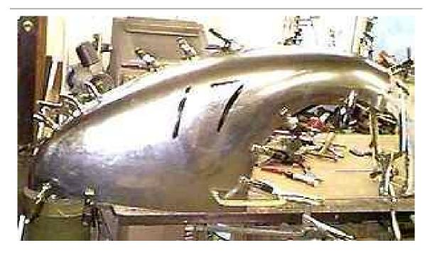
The panel is starting to shine up , the wheel imparts it's polished surface to the surface of the panel.
