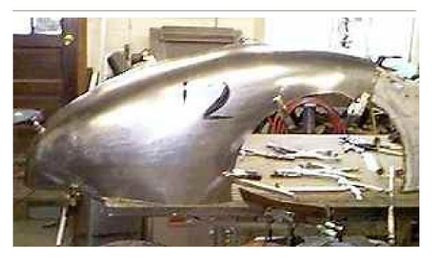
The refinement process continues. A magic marker is used to outline the areas that need raising. In order for the buck to do it's job the panel must be clamped around its outer
