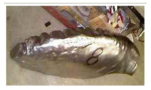
A new series of edge shrinks have been taken to further develope the shape.
