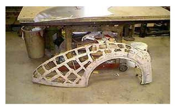
This is my wireform reinforced buck or form which was made by first making a wireform (1/4" dia.hot roll wire)inside of a good original fender. A paste wax was applied to the inside of the original fender, the wireform reinstalled, and then bondo is spread around the wires using a putty knife.
