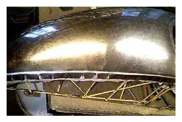
The lower lip of the fender is slowly rolled over with a slapper while it is clamped. Tucks are taken on the inside edge to shrink the inner edge. If the shrinks are not taken, the panel will resist forming.
