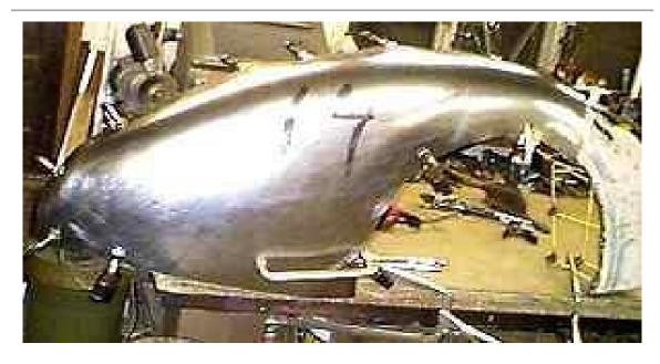
The shape is almost fully developed, all that is left is further refinement, and smoothing.
