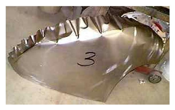
Shrinks have been taken on the edge using a simple tucking tool. By shrinking the edge you develope shape very quickly, but it looks messy.
