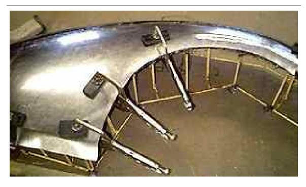
The fender is clamped tightly to the buck and then a wood former is used to reveal the wheel opening joggle and also to start forming the lower lip.
