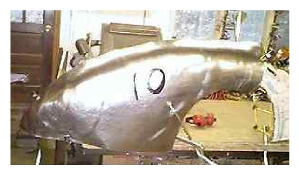
The rough shape is developed and now the buck must be used as a guide to action. By clamping the panel to the buck, low spots will reveal themselves. Low spots are raised by hammering and then wheeling them smooth. At this point minor imperfections in the smoothness of the panel are of no concern. The object is to keep making slight progress on each fitting and adjustment.
