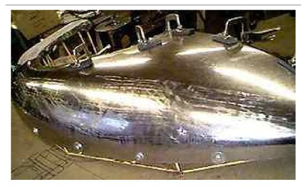
The fender has been bolted to the buck along it's attachment edge. These holes are in the exact location and were copied from the original fender when the buck was made. This type of molded wireform buck allows you to see how the fit is coming, because you have full access to the backside. It also allows you to index or locate and form details in their correct locations. It also allows easy clamping. Clamping zones or pads can be made on the inside of the buck.
