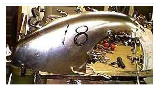
The fender section is now conforming to the buck very well and it is very smooth. The next step is to form the wheel opening joggle and also to turn in the lower rear edge lip, which has a varying radius.
