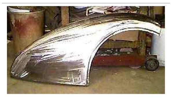
Here's the finished rear fender section. To make the complete fender a front section would
