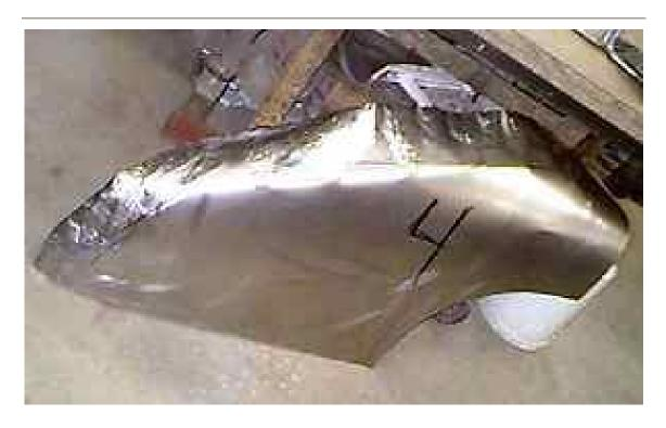
The shrinks have been hammered down (this is all cold working no heat necessary).
