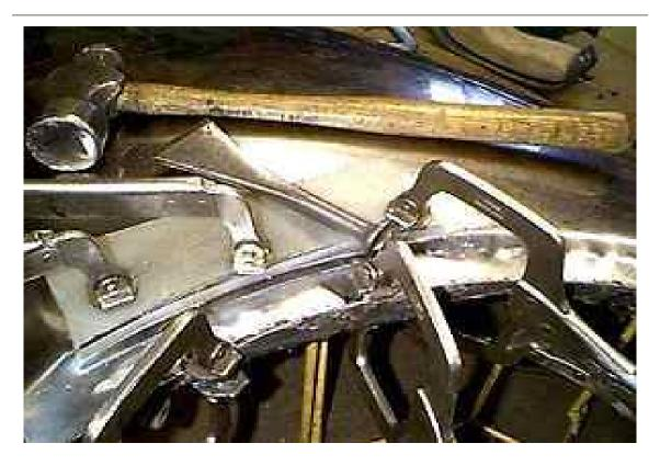
This is a detail shot of the refined joggle. A steel caulking tool is now used to sharpen the inside edge of the joggle.
