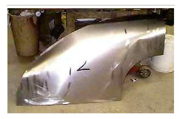
The blank has been rolled on the bench, to make it sort of fit the buck.
