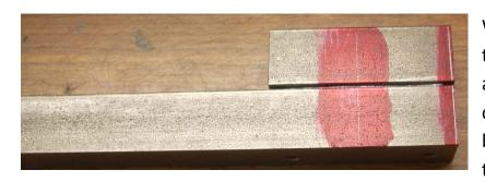
With it all assembled, I then used my Dykem again. I have marked the centerline of the hole to be bored plus how much to clean up at the right
