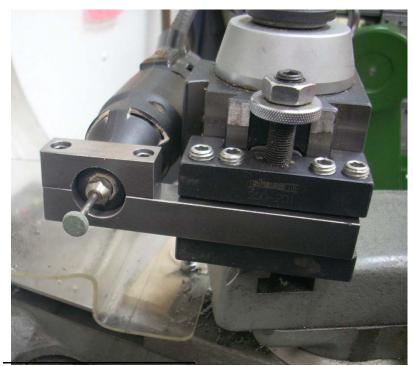
A High Speed Rotary Tool is downright handy at times. And it can be made even more useful if solidly supported in a lathe tool post. Recently I heard this called a "live cutter".
