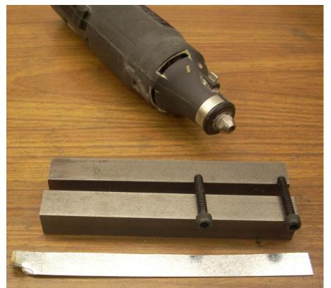
steel (CRS) attached together with a pair of socket head screws. I will call the long bar the support and short bar the clamp.
