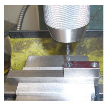
Here you see the two bars lined up. I then raise the drill, remove the clamp bar, and drill through the support bar.
