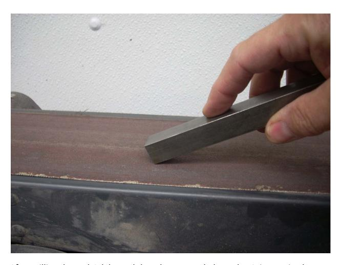
After milling the end, I deburred the edges on my belt sander. It is amazing how well these machines remove metal.
