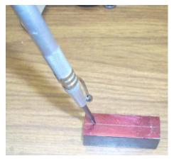
These scribe lines are a little hard to see so I am using a mark out spring loaded punch at each intersection.
