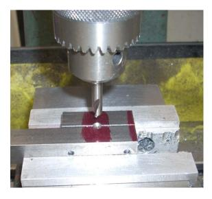
I'm now using my ¼" centering drill to provide a cone shaped hole for my first drill.
