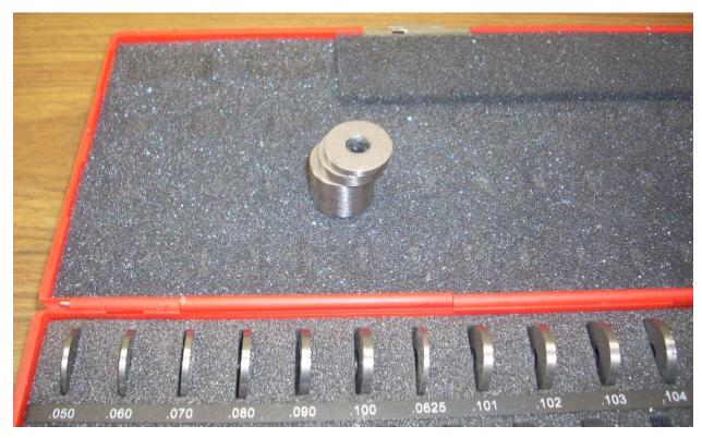
The first step is to have an accurate distance of 0.8750". I own a set of spacer blocks that are good to within +/-0.0001".
