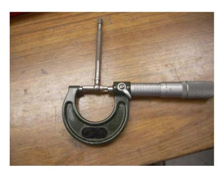
A light touch on the mic is essential. It should go without saying that all surfaces must be free of swarf or grit. This includes the bore.
