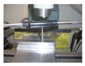
The tap goes in far enough to be secured in the hole. A tap handle can then be attached to finish the job.
