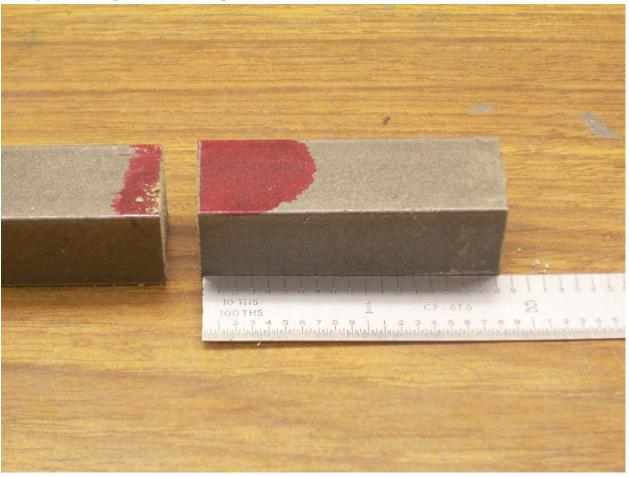
I used my tenth inch ruler to get me close to the 1.85" line. I then used red Dykem® marking fluid to color the area. Then I used a small square and a sharp knife to draw a thin line through the red dye at the desired position. I could have done the measuring right on my bandsaw but wanted you to see the value of marking fluid. After the piece was sawed off, I used my belt sander to remove all burrs from both pieces.
