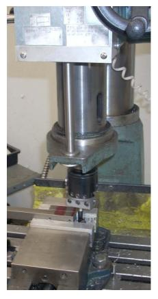
Although not idea from a support standpoint, my boring head will be cutting with the quill all the way down.
