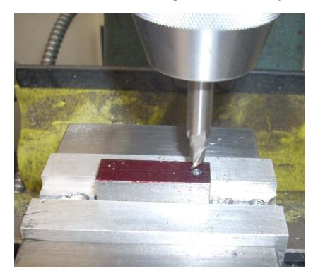
I am using a 2 flute end mill here which can be used to drill holes because it is able to "center cut". A 4 flute end mill cannot typically center cut so would not be a good choice for drilling holes. But since I already have the hole made with the #25 drill, I could use a 4 flute end mill here if I wanted.
