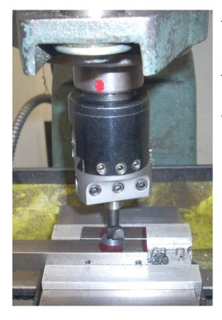
The boring bar is set to just touch the inside of the drilled hole. I want to bore a hole 7/8" in diameter which is 0.8750". This hole does not have to be very precise but I need the practice so will do the best I can. This means being able to know when I'm at the correct diameter.
