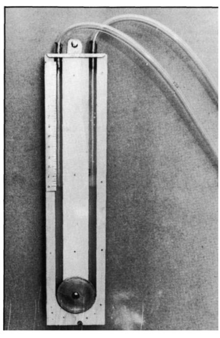
Dynamic pressure minus static pressure is velocity pressure. When one leg of the water gauge is connected to a port to read dynamic pressure and the other leg is connected to a port to read the static pressure, the velocity pressure can be read directly from the manometer. The static pressure and dynamic pressure oppose each other. The difference, velocity pressure, is, in a sense, calculated within the gauge.
